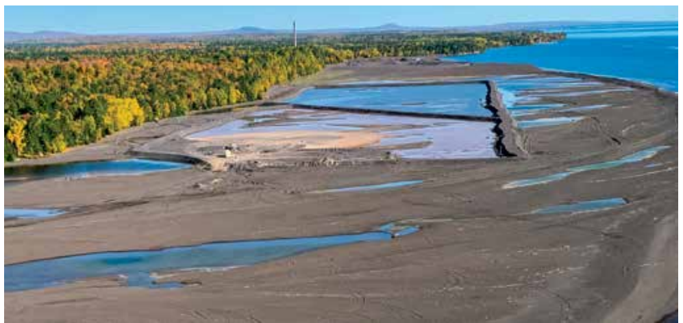
Looking north toward the village of Gay, Michigan, dark-colored stamp sands are seen along the shoreline of Lake Superior in October 2019. The stamp sands are tailings from historic copper stamp mill operations from the Mohawk and Wolverine mines. Photo: Neil Harri, Michigan Department of Natural Resources
